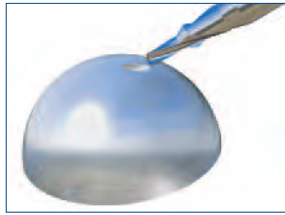
Inclined holes on convex surfaces
